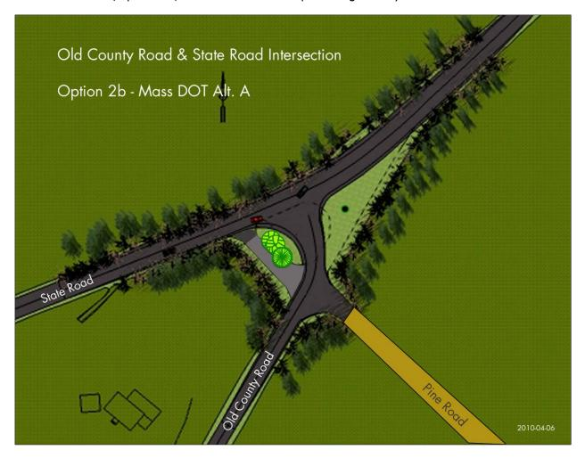
2.4 Possibility of Left-Turn Lane on Old County Road: The level of service analysis showed that the introduction of a left-turn lane on State Road would not have a significant impact on delays on State Road. However, it shows that the delay for vehicles turning onto State Road from the north end of Old County Road is already more than 19 seconds and is projected to increase to 29 seconds.
