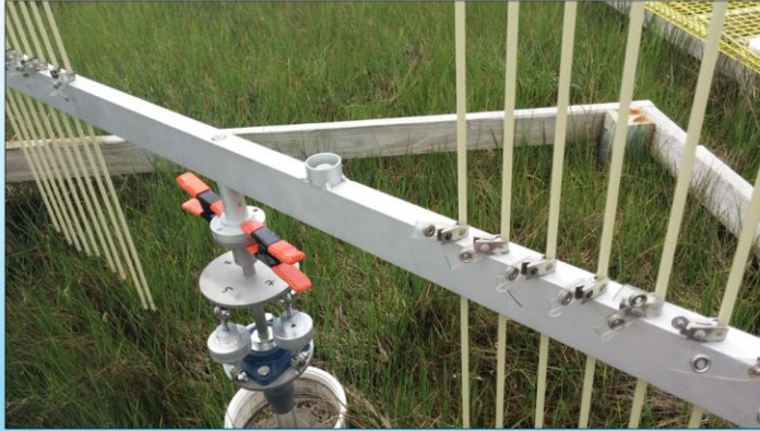
Rod-SET Survey Armature Measures Elevation Edey Foundation Purchased the Armature
